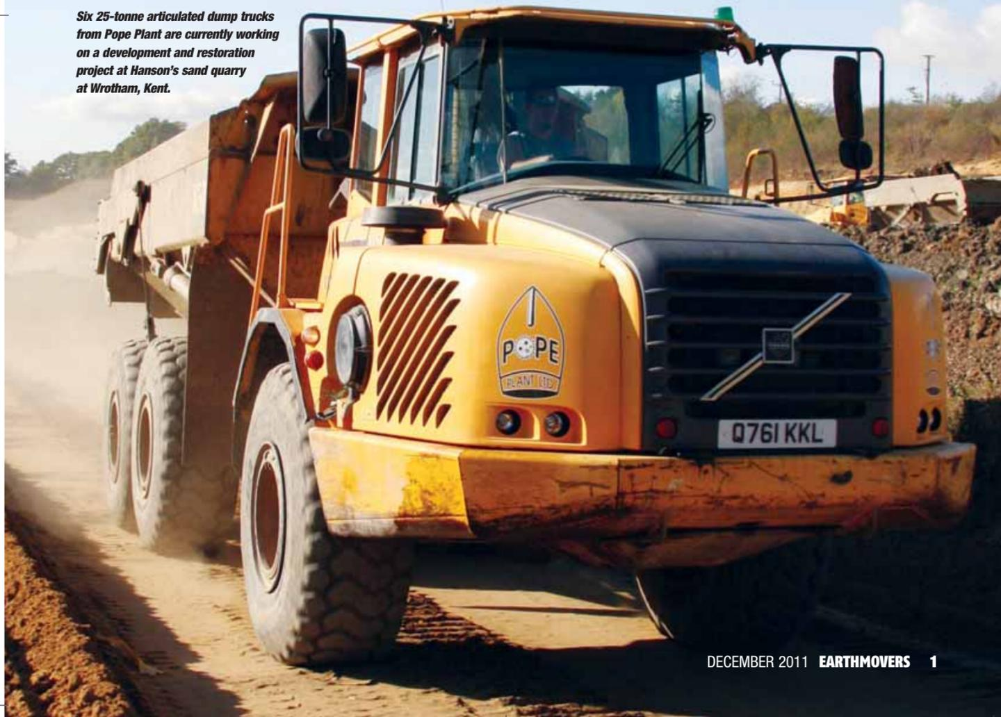
**Older Volvo A25C articulated dump trucks are still providing sterling service, despite having a few hours on the clock and being worked hard on this site.**
